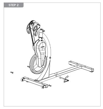
Attach the DRIVE FRAME to the BASE FRAME using 8mm ALLEN KEY WRENCH and item 1-FLAT WASHER and item 2-SOCKET HEAD CAP SCREW.
