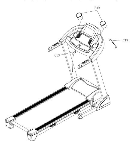
**Step 6:** To check if the running belt runs correctly, placing treadmill in folding position and tightening all the bolts. Then set speed under 3km/h and see if running belt runs without problem.
