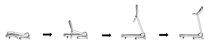
**STEP 3:** According to the picture, tighten the bottom frame with bolt M8\*45(D16) and inner washer(D17). Then locked the console frame with M8\*15 (D13) and inner washer (D17).
